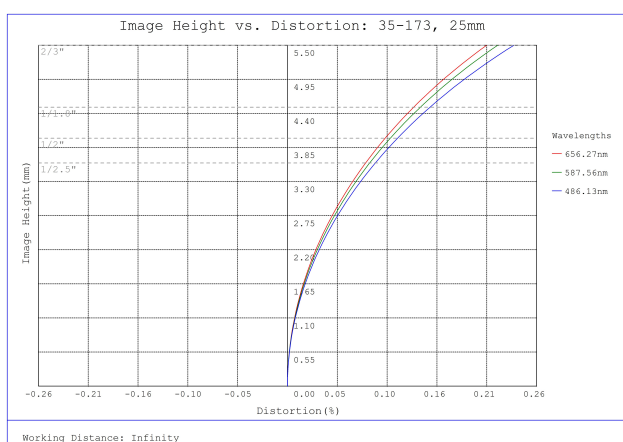
#35-173, 25mm, f/1.8 Cr Series Fixed Focal Length Lens, Distortion Plot
