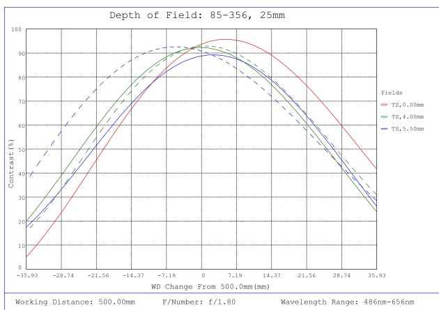
#85-356, 25mm, f/1.8 Ci Series Fixed Focal Length Lens, Depth of Field Plot, 500mm Working Distance, f1.8
