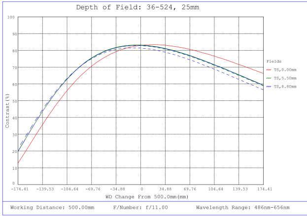
#36-524, 25mm f/11.0, HPr Series Fixed Focal Length Lens, Depth of Field Plot, 500mm Working Distance, f11
