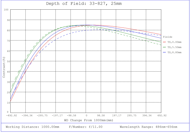
#33-827, 25mm f/11.0, HPI Series Fixed Focal Length Lens, Depth of Field Plot, 1000mm Working Distance, f11
