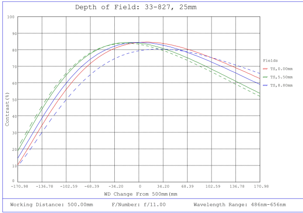
#33-827, 25mm f/11.0, HPI Series Fixed Focal Length Lens, Depth of Field Plot, 500mm Working Distance, f11
