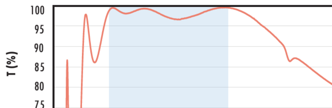
Fused Silica with YAG-BBAR Coating Typical Transmission
