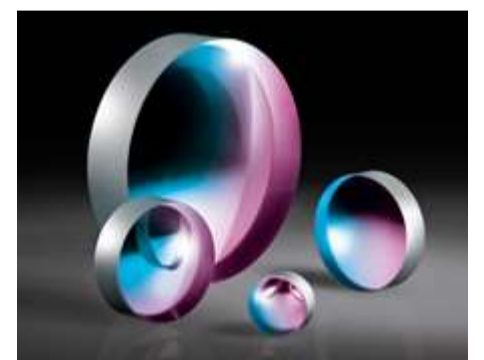
#48-051 - 12.0mm Dia. x -30 FL, UV-AR Coated, UV Plano-Concave Lens ₹15,840
