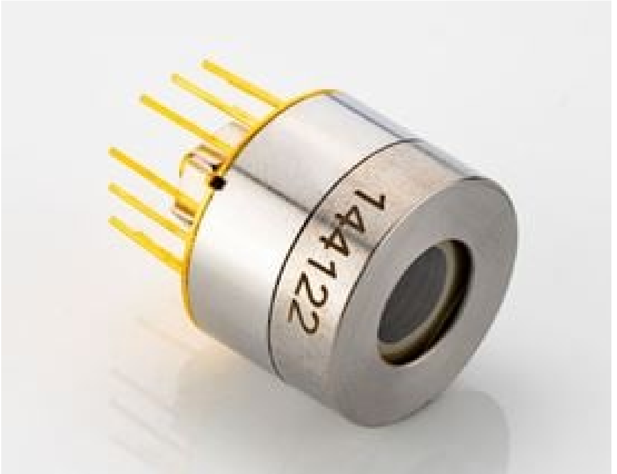
2.3 - 4.4um HgCdTe Photovoltaic Infrared Detector, PVI-2TE-4-1x1-TO8-wAl203-36
