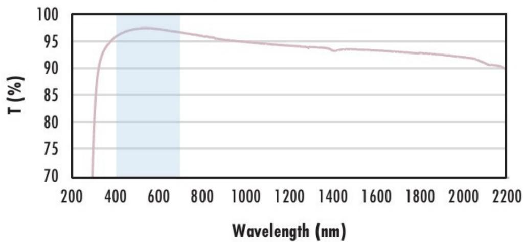
Typical transmission of a 3mm thick N-BK7 window with MgF<sub>2</sub> (400-700nm) coating at 0° AOI.
