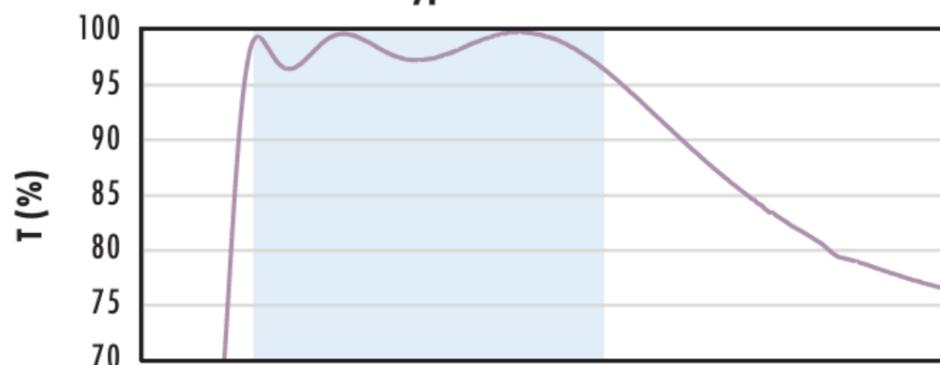
Typical transmission of a 3mm thick N-BK7 window with VIS-NIR (400-1000nm) coating at 0° AOI.
