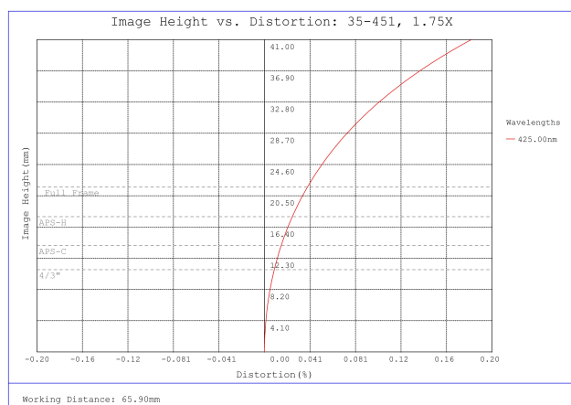
#35-451, 1.75X LS Series Area Scan Lens, Distortion Plot
