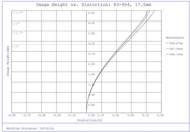
#83-954, 17.5mm FL f/8, Blue Series M12 Lens, Distortion Plot
