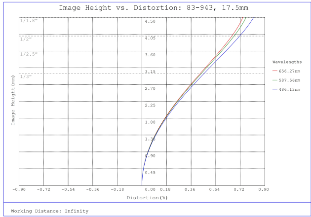
#83-943, 17.5mm FL f/5.6, Blue Series M12 Lens, Distortion Plot
