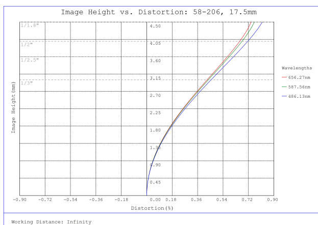
#58-206, 17.5mm FL f/2.5, Blue Series M12 Lens, Distortion Plot
