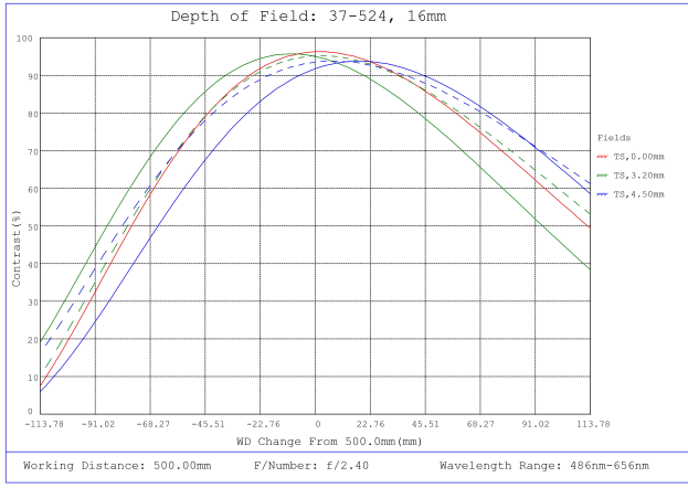
#37-524, 16mm FL, Liquid Lens M12 Lens, Depth of Field Plot, 500mm Working Distance, f2.4
