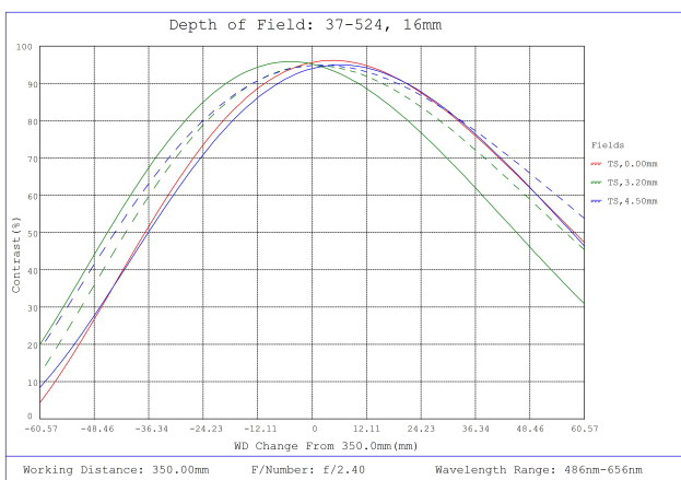
#37-524, 16mm FL, Liquid Lens M12 Lens, Depth of Field Plot, 350mm Working Distance, f2.4
