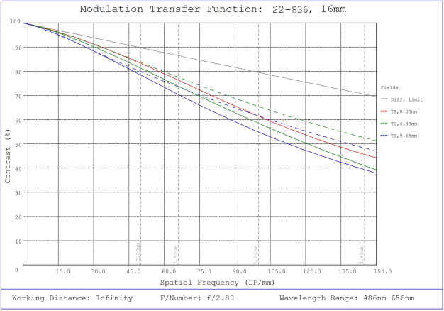
#22-836 - 16mm Focal Length, UAV Series Fixed Focal Length Lens, Modulated Transfer Function (MTF) Plot, Infinity Working Distance, f2.8
