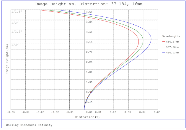
#37-184, 16mm FL f/8.0 Blue Series M12 Lens, Distortion Plot
