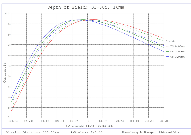
#33-885, 16mm, f/4 UCI Series Fixed Focal Length Lens, Depth of Field Plot, 750mm Working Distance, f4
