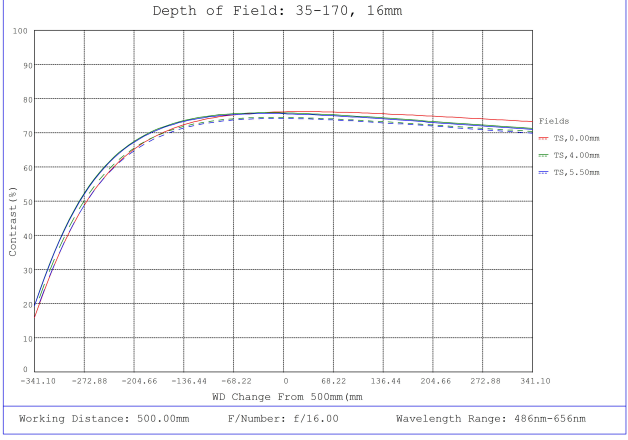
#35-170, 16mm, f/16 Cr Series Fixed Focal Length Lens, Depth of Field Plot, 500mm Working Distance, f16
