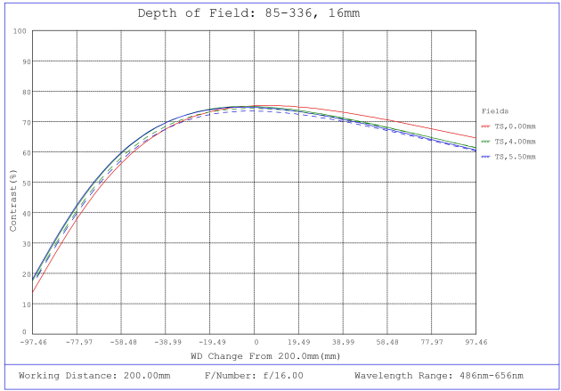
#85-336, 16mm, f/16 Ci Series Fixed Focal Length Lens, Depth of Field Plot, 200mm Working Distance, f16
