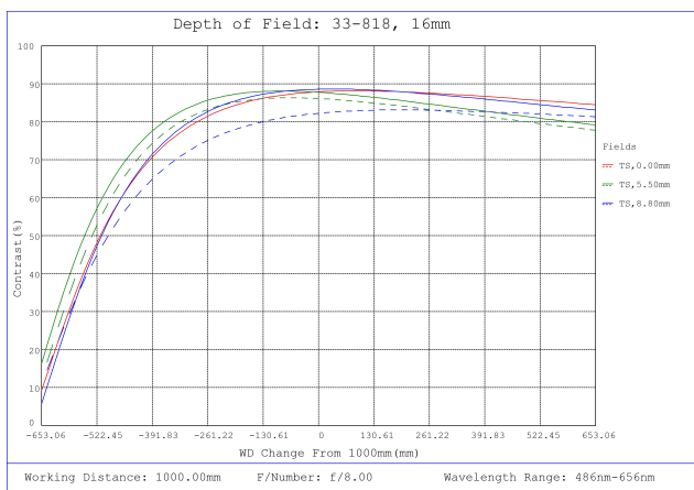
#33-818, 16mm f/8, HPI Series Fixed Focal Length Lens, Depth of Field Plot, 1000mm Working Distance, f8
