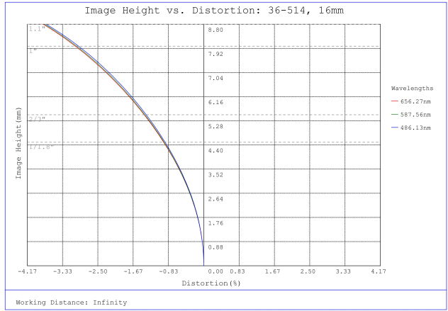
#36-514, 16mm f/5.6, HPr Series Fixed Focal Length Lens, Distortion Plot
