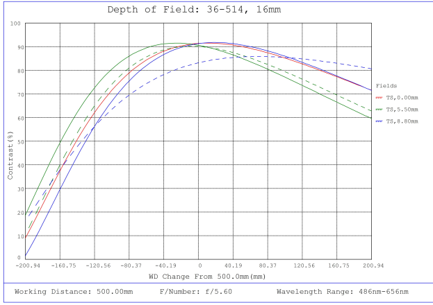
#36-514, 16mm f/5.6, HPr Series Fixed Focal Length Lens, Depth of Field Plot, 500mm Working Distance, f5.6
