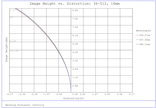
#36-512, 16mm f/2.8, HPr Series Fixed Focal Length Lens, Distortion Plot
