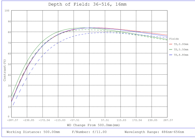
#36-516, 16mm f/11, HPr Series Fixed Focal Length Lens, Depth of Field Plot, 500mm Working Distance, f11
