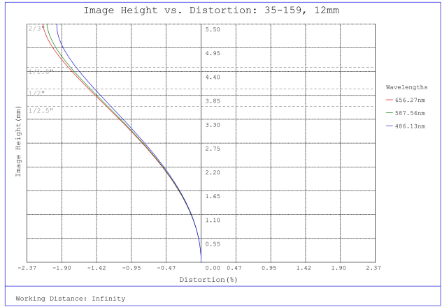
#35-159, 12mm, f/8 Cr Series Fixed Focal Length Lens, Distortion Plot
