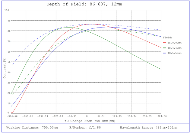
#86-607, 12mm, f/1.8 Ci Series Fixed Focal Length Lens, Depth of Field Plot, 750mm Working Distance, f1.8
