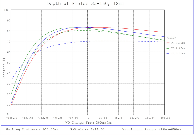
#35-160, 12mm, f/11 Cr Series Fixed Focal Length Lens, Depth of Field Plot, 300mm Working Distance, f11
