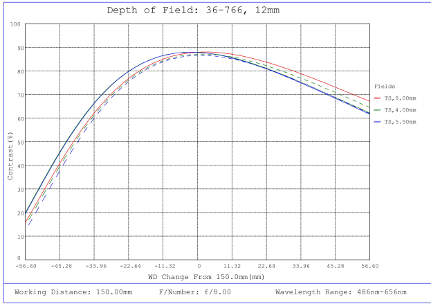
#36-766, 12mm f/8, 150-500mm Primary WD, HRi Series Fixed Focal Length Lens, Depth of Field Plot, 150mm Working Distance, f8
