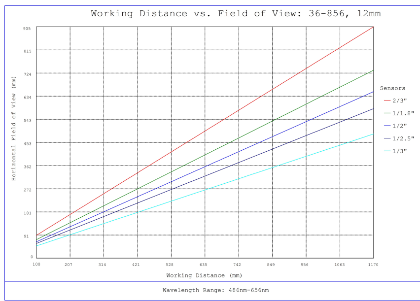
#36-856, 12mm f/5.6, 400-2000mm Primary WD, HRr Series Fixed Focal Length Lens, Working Distance versus Field of View Plot
