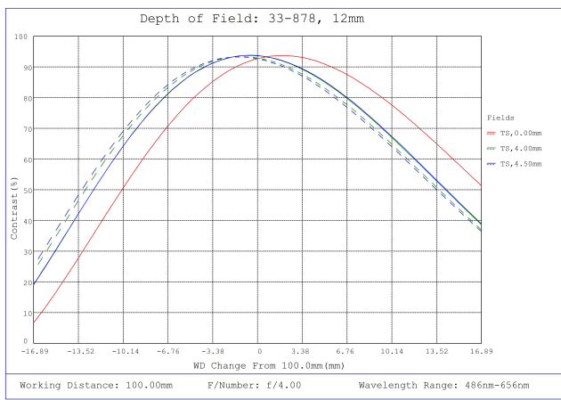
#33-878, 12mm, f/4 UCi Series Fixed Focal Length Lens, Depth of Field Plot, 100mm Working Distance, f4
