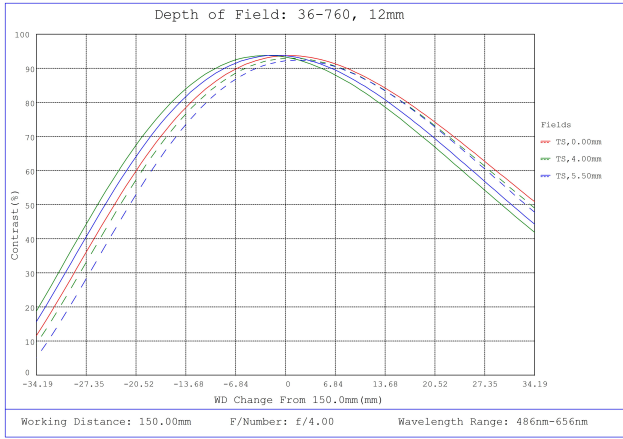
#36-760, 12mm f/4, 150-500mm Primary WD, HRi Series Fixed Focal Length Lens, Depth of Field Plot, 150mm Working Distance, f4
