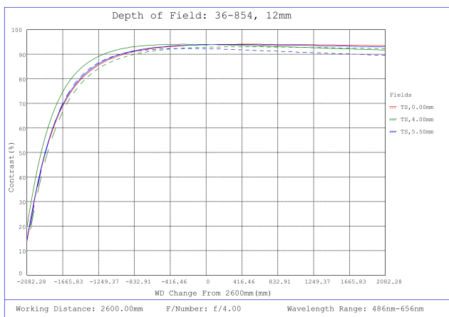
#36-854, 12mm f/4, 1000mm-∞ Primary WD, HRr Series Fixed Focal Length Lens, Depth of Field Plot, 2600mm Working Distance, f4
