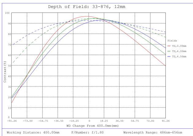
#33-876, 12mm, f/1.8 UCi Series Fixed Focal Length Lens, Depth of Field Plot, 400mm Working Distance, f1.8
