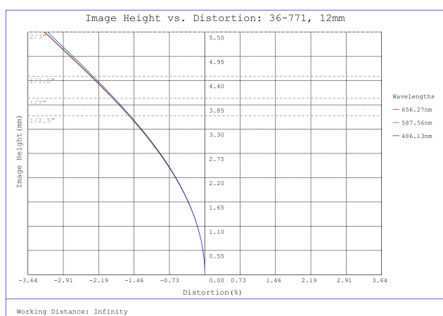
#36-771, 12mm f/11, 1000mm-∞ Primary WD, HRi Series Fixed Focal Length Lens, Distortion Plot
