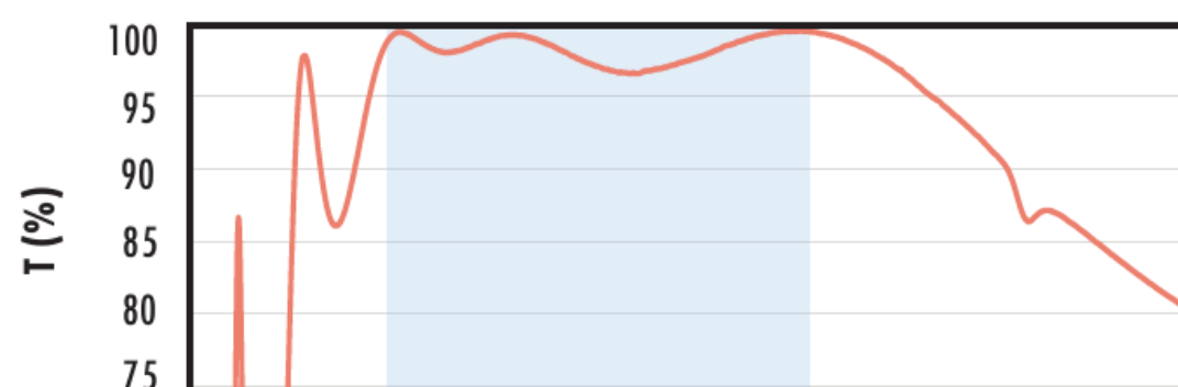
Fused Silica with YAG-BBAR Coating Typical Transmission
