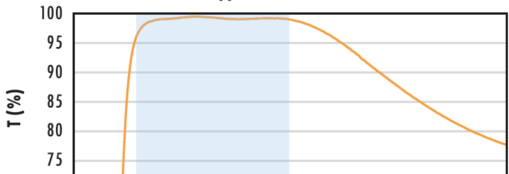
N-BK7 with VIS-EXT Coating Typical Transmission
