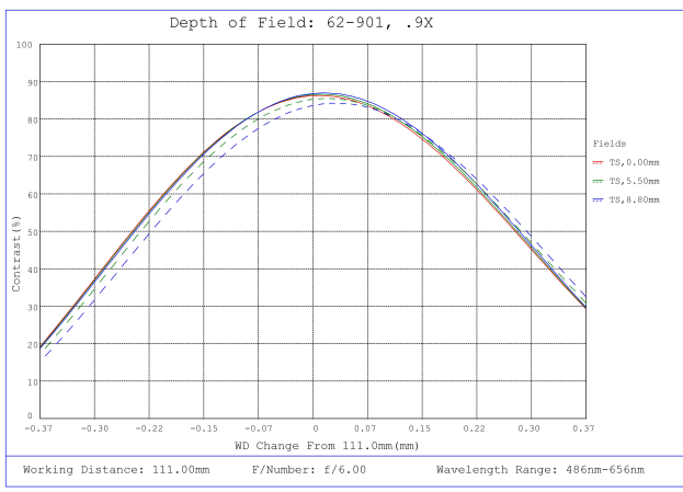
#62-901, 0.9X CobaltTL Telecentric Lens, Depth of Field Plot, 111mm Working Distance, f6
