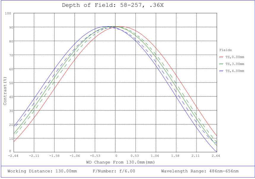
#58-257, 0.36X ½" GoldTL™ Telecentric Lens, Depth of Field Plot, 130mm Working Distance, f6
