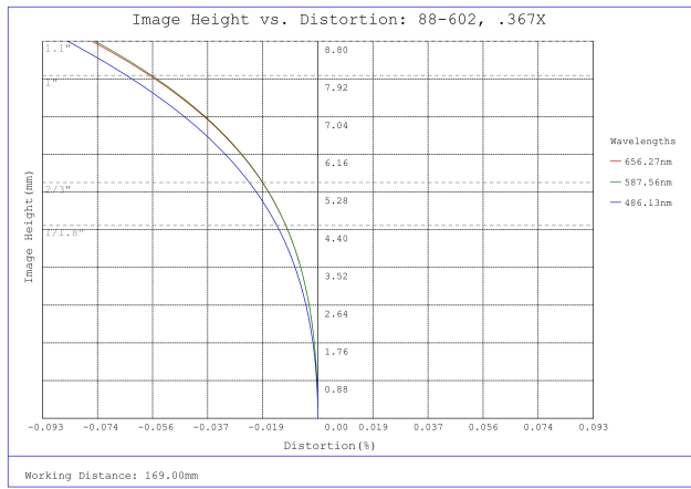
#88-602, 0.367X CobaltTL Telecentric Lens, Distortion Plot
