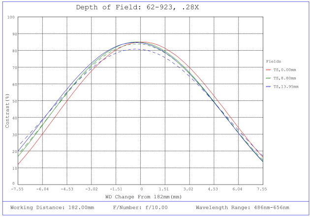
#62-923, 0.28X, 28.7mm M42 x 1.0 (6.56mm) PlatinumTL™ Telecentric Lens, Depth of Field Plot, 182mm Working Distance, f10
