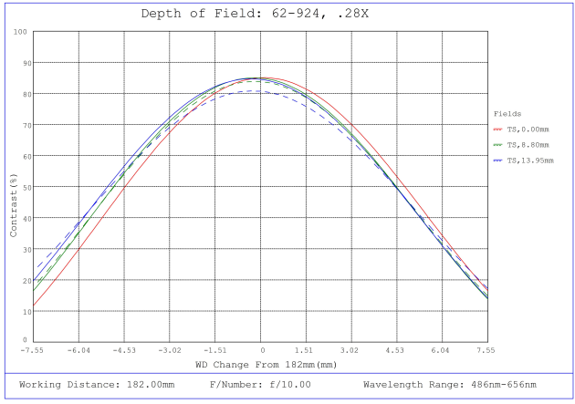
#62-924, 0.28X, 28.7mm M42 x 1.0 (19.53mm) PlatinumTL™ Telecentric Lens, Depth of Field Plot, 182mm Working Distance, f10
