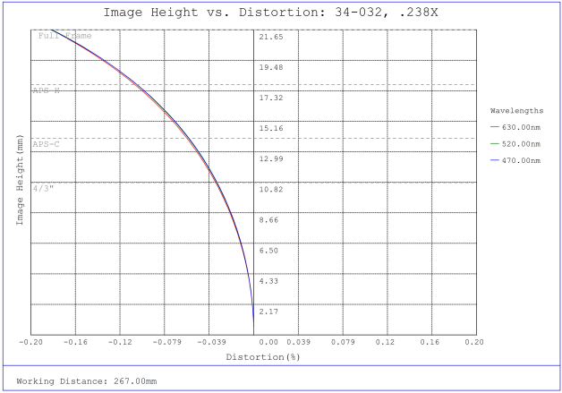
#34-032, 0.238X, 35mm F-Mount TitanTL® Telecentric Lens, Distortion Plot
