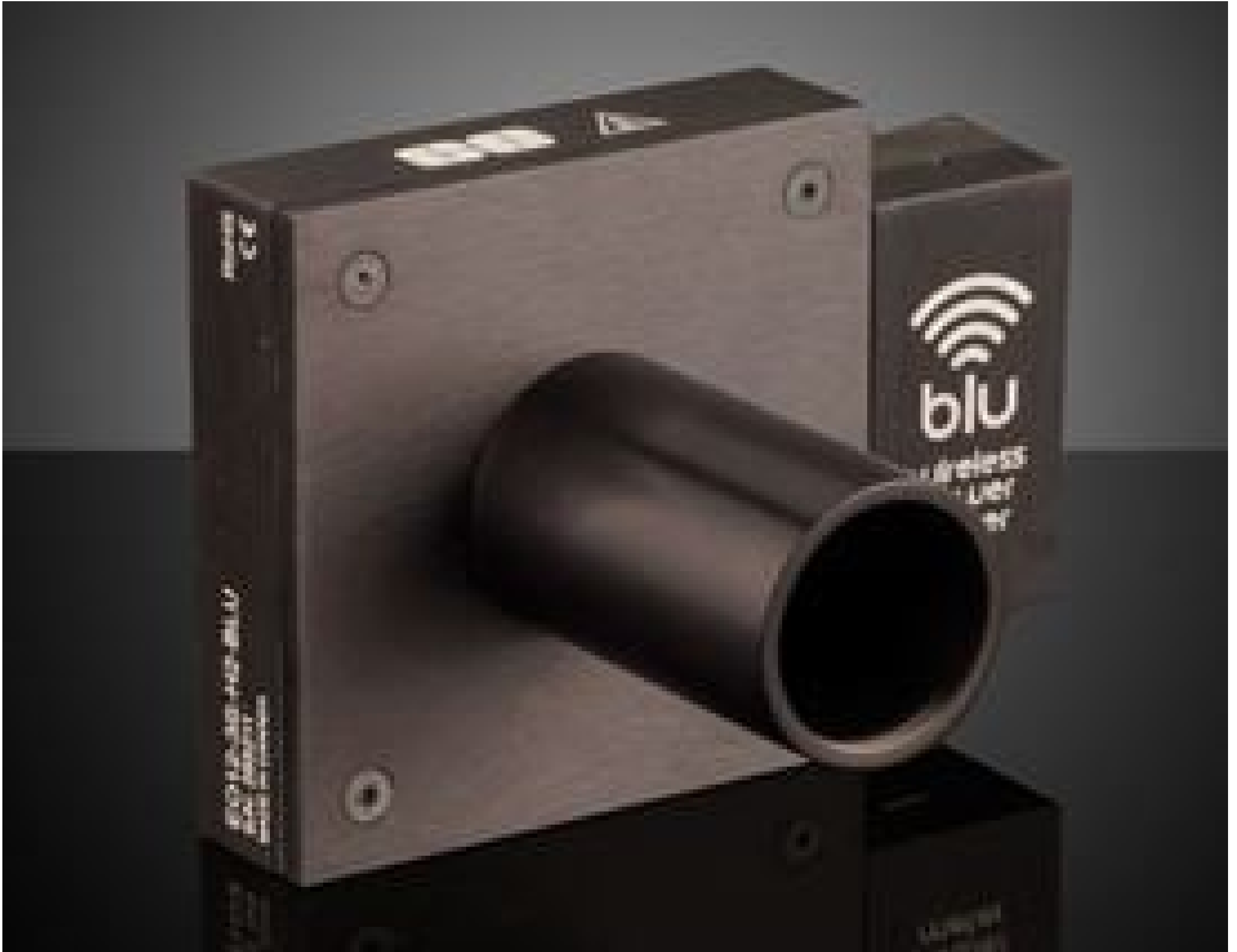
0.19 - 20 \mu m, 3W, Thermopile Wireless Power Detector
