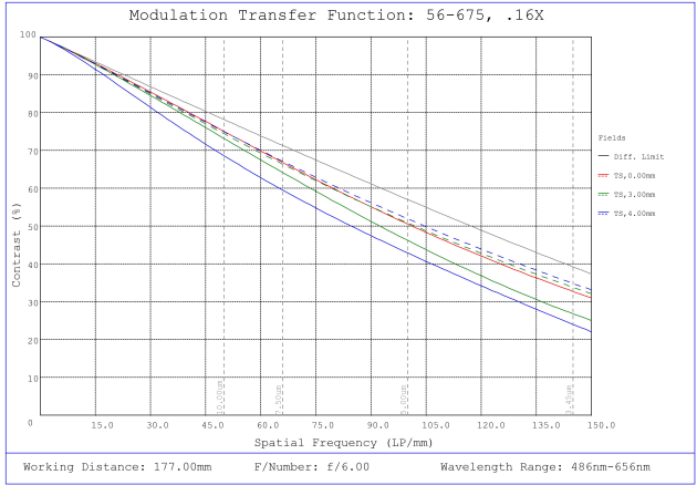
#56-675, 0.16X SilverTL™ Telecentric Lens, Modulated Transfer Function (MTF) Plot, 177mm Working Distance, f6
