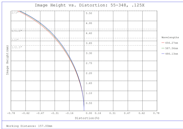
#55-348, 0.125X, 2/3" GoldTL™ Telecentric Lens, Distortion Plot
