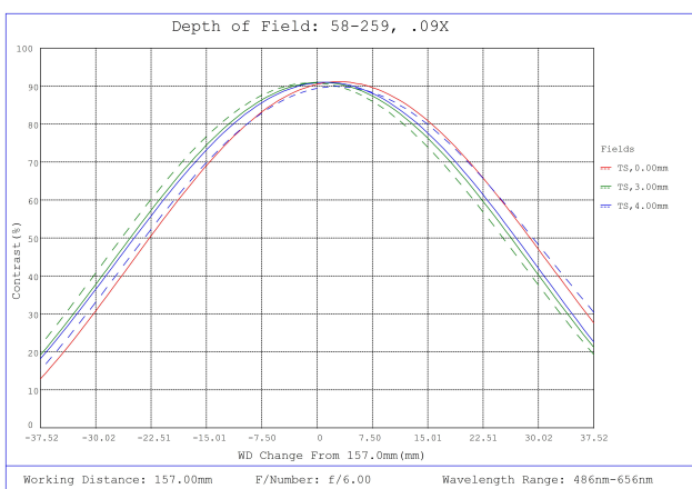
#58-259, 0.09X 1/2" GoldTL™ Telecentric Lens, Modulated Transfer Function (MTF) Plot, 157mm Working Distance, f6
