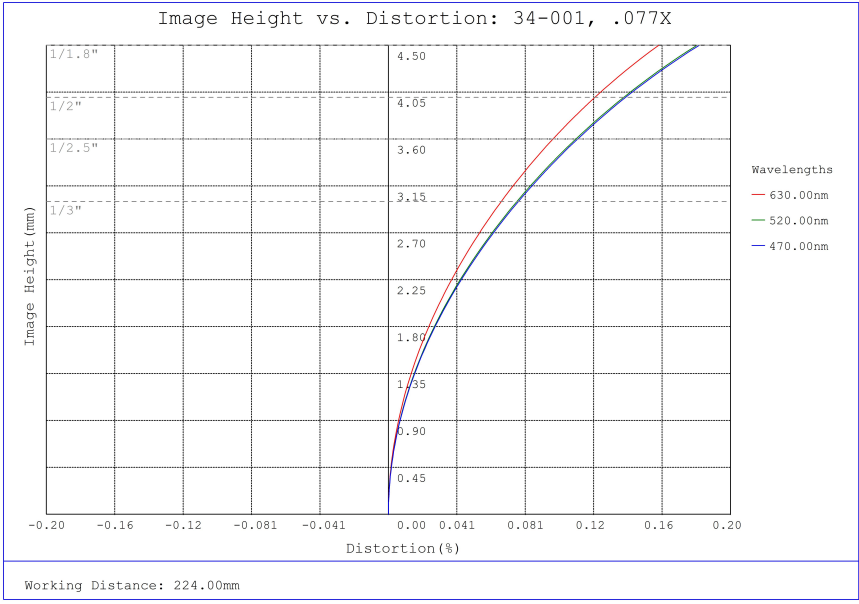
#34-001, 0.077X, 1/1.8" C-Mount TitanTL® Telecentric Lens, Distortion Plot
