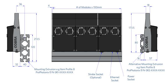
For all COBRA MultiSpec longer than 100-mm, standard item brand aluminum extrusion Profile 8 is used for rigidly aligning and connecting the 100-mm COBRA MultiSpec modules together. The extrusion is also used for mounting of the COBRA MultiSpec. Two options are available (see dimensional specifications).
