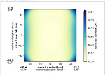
spot diameter at 86.5% level for a Gaussian beam ( $M^2$  = 1) with 12.0 mm diameter at  $1/e^2$ , clipped at 12.0 mm field size and mirror distances as given above for a two mirror scan system
