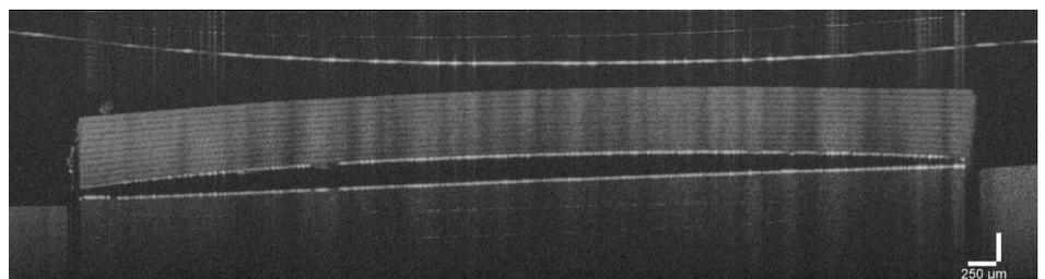
OCT test system specifications: Spectral Domain OCT Imaging System, 1300 nm, axial resolution is 5.5 microns, lateral resolution of 13 microns.
